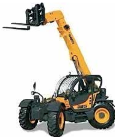
Service Rentals' Dieci Reach Forklift unit comes with a load sensor.
